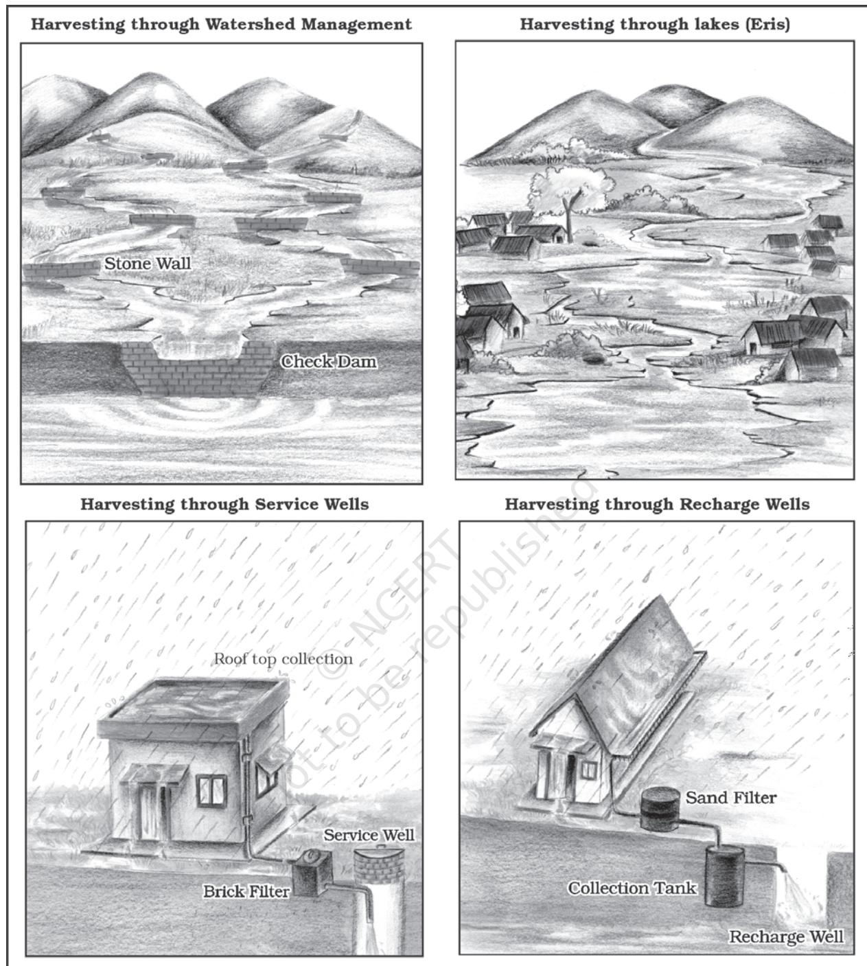
**Fig. 6.3 : Various Methods of Rainwater Harvesting**
